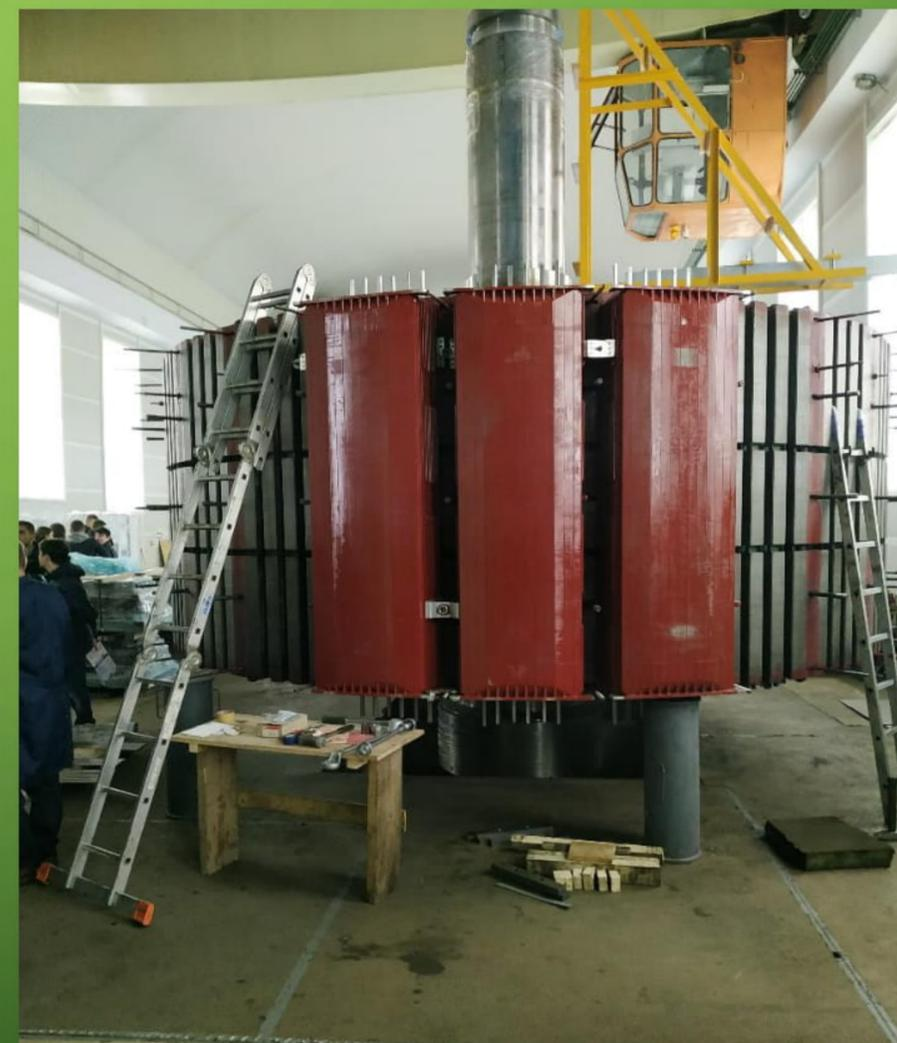
Sinhroni hidrogenerator, 120 MVA,  $\cos\varphi=0.95$ , 15.75 kV,
